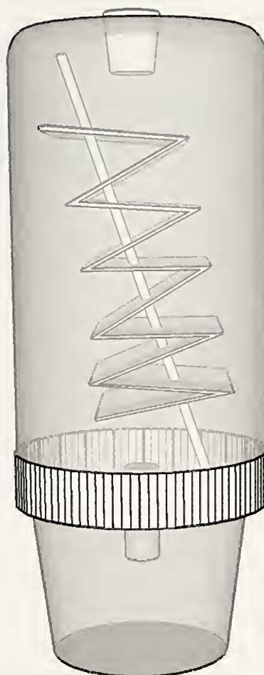
Figure 1.—Salticid maintenance cage. Each cage (diameter 55 mm, height 100 mm) contained a piece of dark cardboard folded in a bellows shape kept in place by a thin bamboo stick pierced through the cardboard folds. A hole in the top was used for introducing prey. Water provided via cotton wick partially immersed in water and extending through base of cage.
